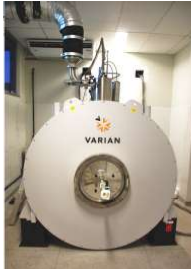
FIGURE 3: 7 TESLA, 210 BORE ACTIVELY SCREENED REFRIGERATED MAGNET SYSTEM. VARIAN, INC. NMR SYSTEMS. PROFESSOR IN CHARGE: FERNANDA TOVAR MOLL.
