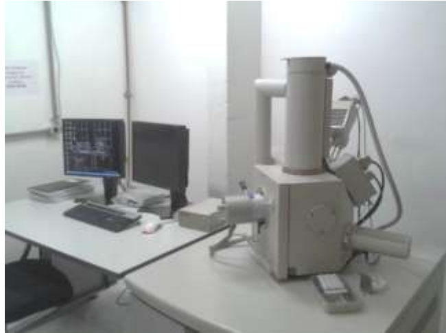
FIGURE 14: SCANNING ELECTRON MICROSCOPE QUANTA 250, FEI COMPANY BRAND. TENSION BETWEEN 1-30 KV, EQUIPPED WITH A PELTIER SAMPLE COOLER (ENVIRONMENTAL MODE) AND BEAM DECELERATOR. ABLE TO WORK IN HIGH (10 -2 A 10 -4 PA), LOW VACUUM (10 A 130 PA) AND ENVIRONMENTAL MODE(10, 400 PA), ALLOWING THE OBSERVATION OF NON-CONDUCTIVE AND / OR HYDRATED MATERIALS. HAS AN X-RAY DETECTOR FOR ELECTRON MICROANALYSIS AND MAPPING, AND A DETECTOR OF BACKSCATTERED ELECTRONS AND SECONDARY ELECTRONS. PROFESSOR IN CHARGE: KILDARE MIRANDA. TECHNICIANS: RACHEL RACHID AND THIAGO LUIZ DE BARROS MOREIRA.
