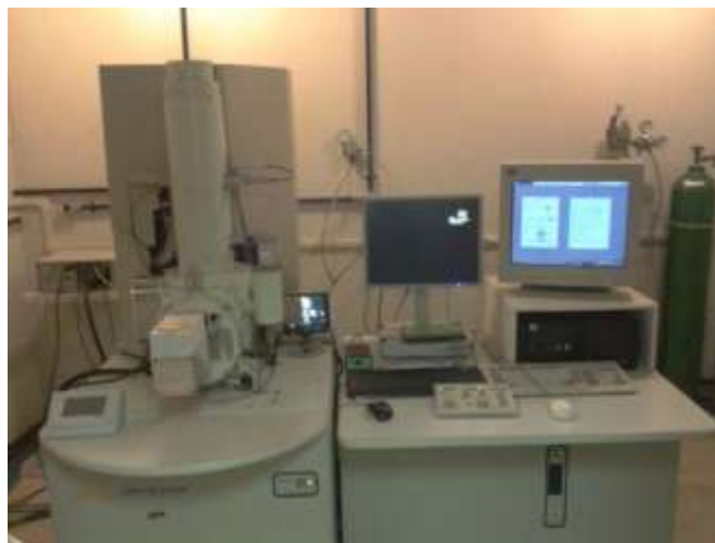
FIGURE 9: SCANNING ELECTRON MICROSCOPE JEOL JSM 6340, HIGH RESOLUTION WITH FIELD EMISSION GUN. EQUIPPED WITH CRYO-STAGE, DETECTOR OF BACKSCATTERED ELECTRONS AND SECONDARY ELECTRONS. PROFESSOR IN CHARGE: KILDARE MIRANDA. TECHNICIANS: DANIEL IUCIF AND THIAGO LUIZ DE BARROS MOREIRA.
