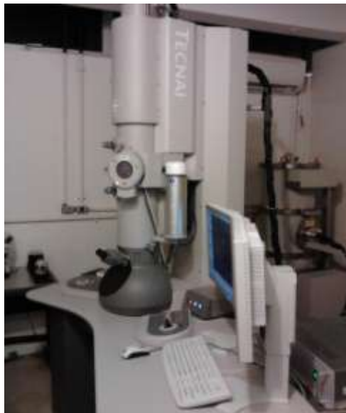
FIGURE 13: TRANSMISSION ELECTRON MICROSCOPE TECNAI G20, D2114, FEI COMPANY, OPERATING AT 200 KV. EQUIPPED WITH TOMOGRAPHY HOLDER, ABLE TO OBTAIN IMAGES AROUND ITS Y AXIS, AT THE ANGULAR RANGE OF -70^{\circ} TO +70^{\circ} . CONFIGURED FOR ELECTRON TOMOGRAPHY OF BIOLOGICAL SPECIMENS 200-300 NM THICK AND ALLOWS THE ACQUISITION OF TOMOGRAPHIC SERIES FOR ALIGNMENT AND 3D RECONSTRUCTION IN SPECIFIC SOFTWARES. PROFESSOR IN CHARGE: KILDARE MIRANDA. TECHNICIAN: THIAGO LUIZ DE BARROS MOREIRA.
