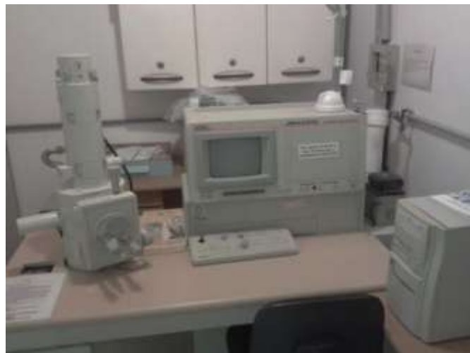
FIGURE 8: SCANNING ELECTRON MICROSCOPE JEOL JSM 5310, WITH MAXIMUM VOLTAGE 25 KV, MAGNIFICATION RANGE FROM 35 TO 100,000 X. PROFESSOR IN CHARGE: KILDARE MIRANDA. TECHNICIANS: NOÉMIA RODRIGUES AND THIAGO LUIZ DE BARROS MOREIRA.
